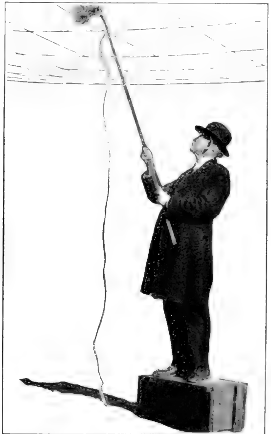
This is not a mop, which Prof. Thordarson is holding. Sparks are leaping to the top of a pole in his hand. From the safety-screen high-voltage charges and thunder-claps are coming
